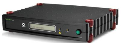
**NeurOne Tesla brings NeurOne technology to MRI field** - Faster sampling and 24 bit resolution as well as MRI synchronized data acquisition. Same Multi Syncbox technology that allows recordings up to 1200 channels with NeurOne Brainstorm.
